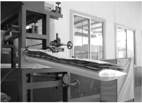
图 3 充气机翼载荷试验 Fig.3 Loading test for the inflatable wing
